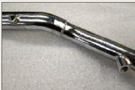
Dual O2 sensor bungs allow for fitment on either '09 or '10 motorcycles. They also offer a convenient way to sample air/fuel ratios without removing the bike's O2 sensors by utilizing the unused bungs.
