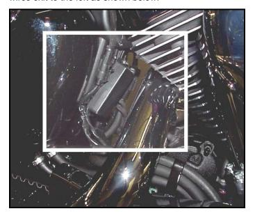
**Step 2d** Insert AutoTune power/communication 4-pin plug into the bike's data port (gray), located at the base of the battery. Re-install the ECM fuse.
