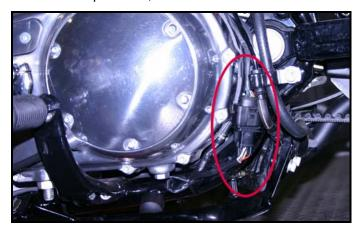
**Step 2g** Rear sensor: Route wiring down the left frame rail behind the primary housing, with the plug located along the frame turn. Double-back the wiring to the rear sensor. Connect the sensor to the closed loop module, secure with wire ties.
